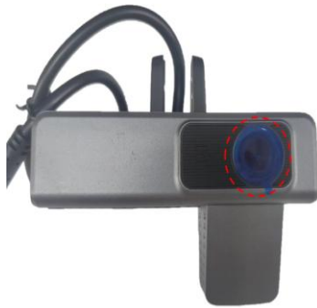
DC-204-AI Rear view showing the road facing lens of the ADAS camera Figure 11
